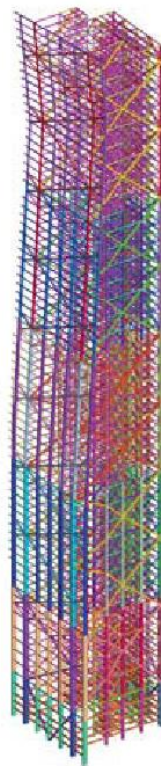
塔楼侧向支撑 Tower Lateral System
